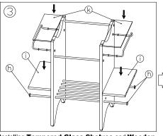
Installing Tempered Glass Shelves and Wooden Adjust and tighten End Caps for fit and fix Wooden
