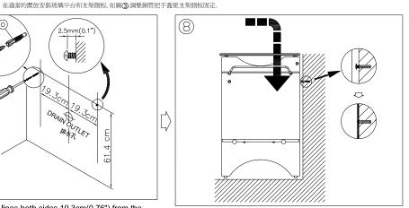
Insert two **Stainless Steel Wall Screw** heads into keyholes on the back of L & R Side Boards and press downward. Be sure the basin table is flush and tighten to wall. ®
