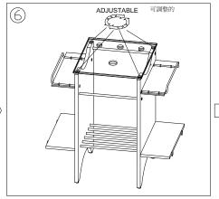
Level Tempered Table Glass by twisting Adjusting Holders.6
