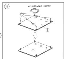
Screwing Adjusting Holders on Tempered Table Glass@
