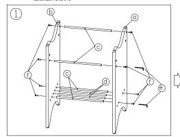
Assembling main parts with attached Hexagon Key as shown in figure 1.
