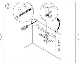
Mark two vertical lines both sides 19.3cm(0.76") from the center of drain outlet, and meantime, using assembled table-keyholes as template or mark and drill two fixing holes for Stainless Steel Wall Screws as shown in figure 7. 用鉛筆在距離牆上排水孔左右各19.3公分處,並在高度61.4公分處畫上2個鎖螺絲的記號, 在畫上記號前,必須注意牆角及地面是否平整且與牆面垂直,並再次確認2記號間與地面
